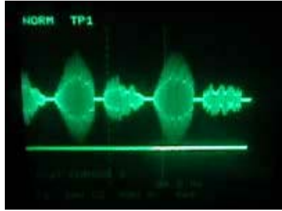
Oscilloscope signal of the multiple-modulated output, load signal in the low frequency domain (carrier is not visible) Frequency, phase, amplitude and PWM multimode-modulation
