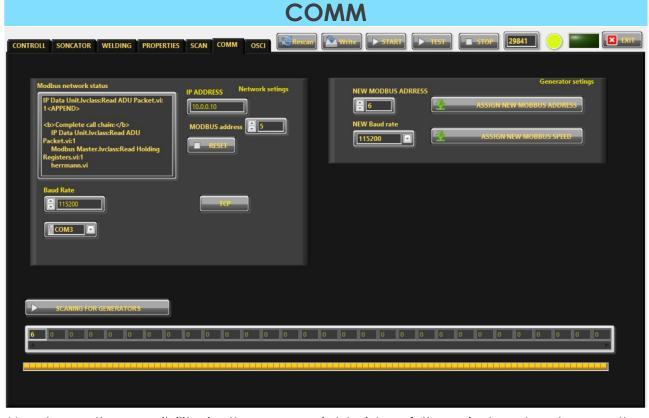
You have the possibility in the upper right side of the window to change the Modbus address selecting a new value in the field "NEW MODBUS ADDRESS" and then press the button "ASSIGN NEW MODBUS ADDRESS".
