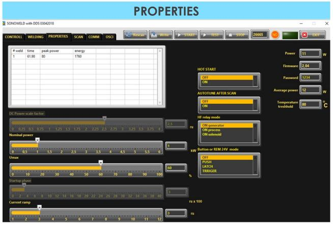
**Current Ramp** - This is a type of regulator of the speed of growing of the current, which starts regulating when Imax is close to the set limit in case when the phase set value is still not reached (in ru). When Current Ramp value is small – the current grows fast, when Current Ramp is big – the current grows slow.
