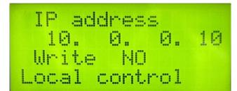
If Local control is selected the generator parameters are available through LCD display.
