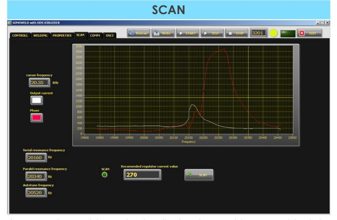
Scan procedure must be made when the transducer and horn are not loaded - operation "on air".
