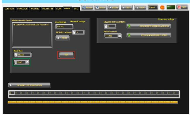
Open the application from Windows menu ("Metal welding 10kW") and go to **COMM** tab. You will notice on the upper right side of the screen an orange circle with NO in it, that means "No connection". Follow the instructions corresponding to the type of connection you made between your PC and the ultrasonic generator.
