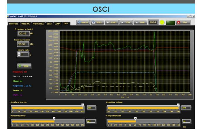
There is an inserted function for recording data – frequency, output current, phase, amplitude and power. Select the duration of the record in the field "time to write" – in seconds. The recording starts of the generator and ends when the selected time to write is finished. After recording is finished, when the button read is pressed, the data from generator is uploaded in the LabView software and is visualized graphically.
