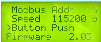
**Modbus Addr** - shows the address of the generator in the Modbus network. The default Modbus Address is 6.
