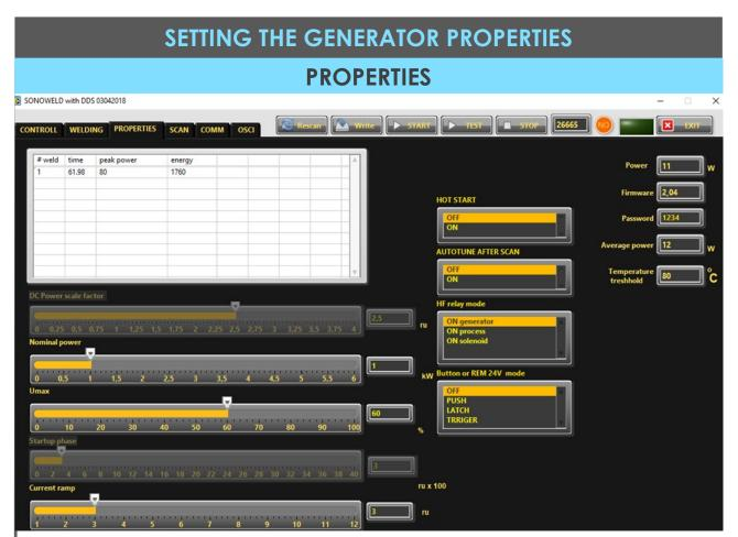
In PROPERTIES Tab you can select the HF Relay Mode (drop down menu) from three options:
