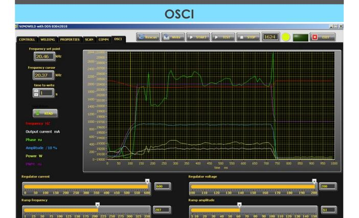
There is an inserted function for recording data – frequency, output current, phase, amplitude and power. Select the duration of the record in the field "time to write" – in seconds. The recording starts by START of the generator and ends when the selected time to write is finished. After recording is finished, when the button read is pressed, the data from generator is uploaded in the LabView software and is visualized graphically.
