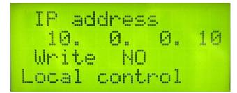
If Local control is selected the generator parameters are available through LCD display **Note:** In both cases USB connection is available.
