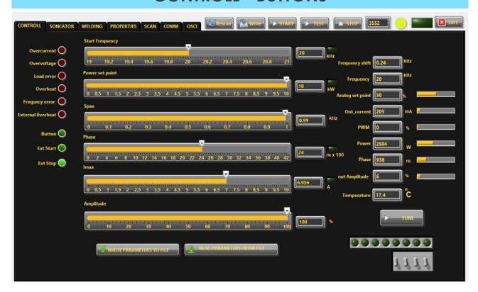
**TUNE -** Starts the auto tuning process. If better starting frequency is found the **Freq** value will be replaced with new one, or else the **Freq** value will remain the same.
