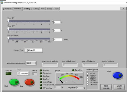
**Time ON** – Set the operation time of the generator in Sonicator mode.
