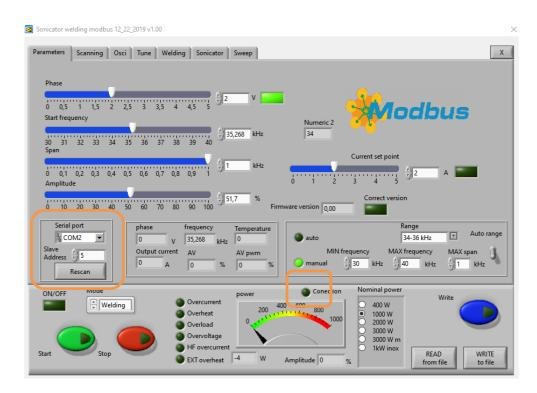
Press "RESCAN". **Connection** (lime-green) light should be blinking. Now you are connected to the generator with the selected address.
