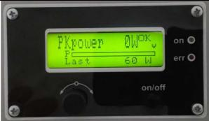
"Welding by limited amount of Energy" which should be sent to a load. Welding process will stop when given amount of Energy is delivered to a load.
