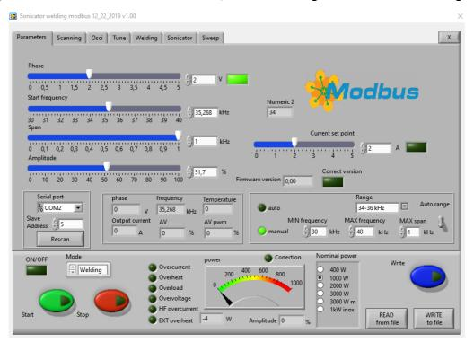
7. After pressing the button RESCAN you have all parameters and settings from the generator uploaded in Labview software.
