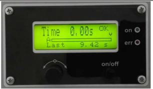
"Welding by limiting the Peak power on the load". Welding process will stop when Peak power is reached.
