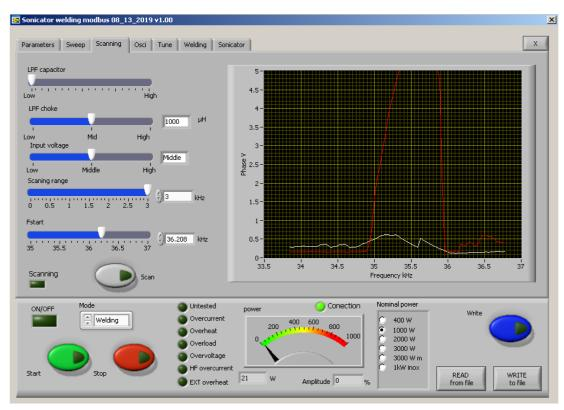
The generator has Scanning function which is very powerful instrument for the operator. Here you can discover the phase and current characteristic of the exact load. It is shown graphically in an window in Scanning tab.
