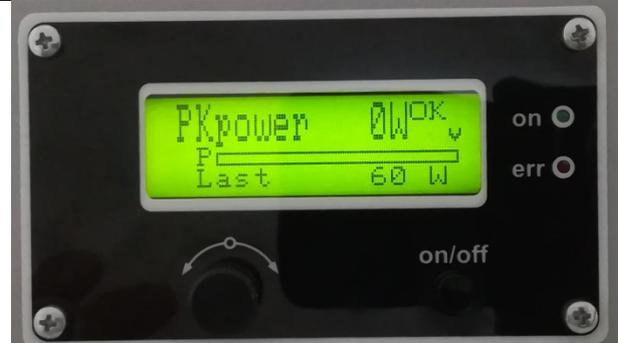
“Welding by limited amount of Energy” which should be sent to a load. Welding process will stop when **given amount of Energy** is delivered to a load.
