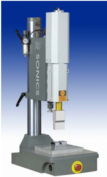
Sonics Model 2055 20 kHz Ultrasonic Welder
