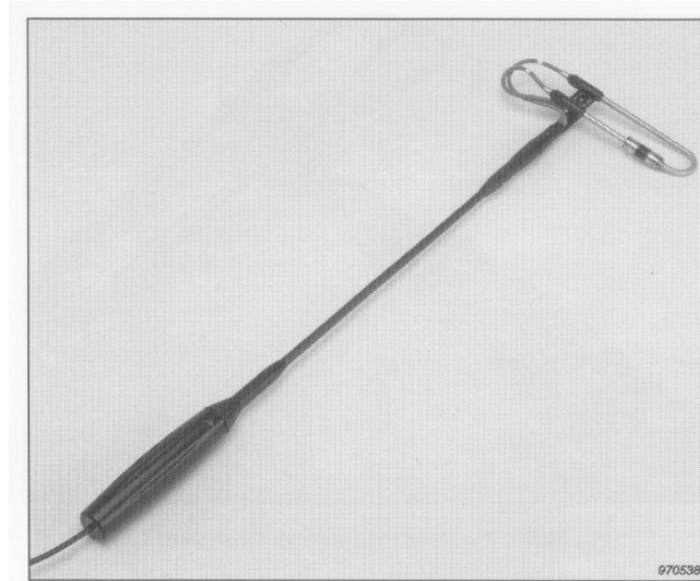
Figure 3.1 Sound intensity probe manufactured by Brüel & Kjær. The microphones are ‘face-to-face’.
