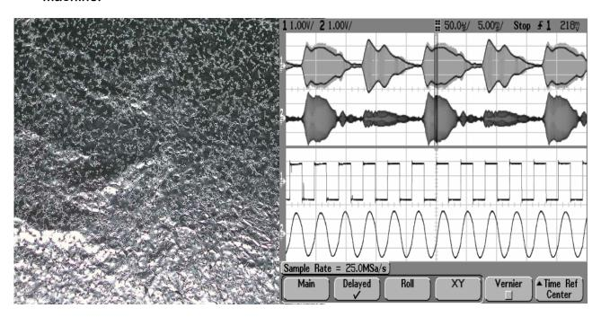
Left: Perfectly, uniformly perforated aluminum foil, after 5 to 10 seconds of exposure to MMM ultrasonic vibrations in an ultrasonic cleaner. Frequency Range: From Hz to MHz; From Infrasonic to Supersonic. Right: Load current and voltage shapes (modulated and carrier).
