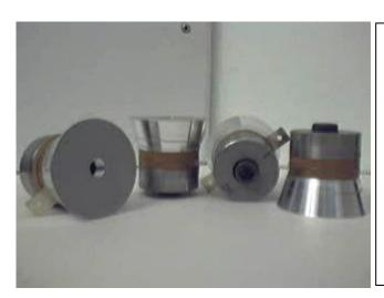
Total axial length = 48 mm, Front mass diameter = 50 mm, h = 19 mm Back mass diameter = 38.5 mm, h = 14 mm
