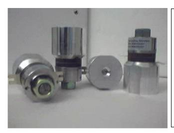
Total axial length = 80 mm, Front mass diameter = 45 mm, h = 39 mm Back mass diameter = 35.5 mm, h = 19
