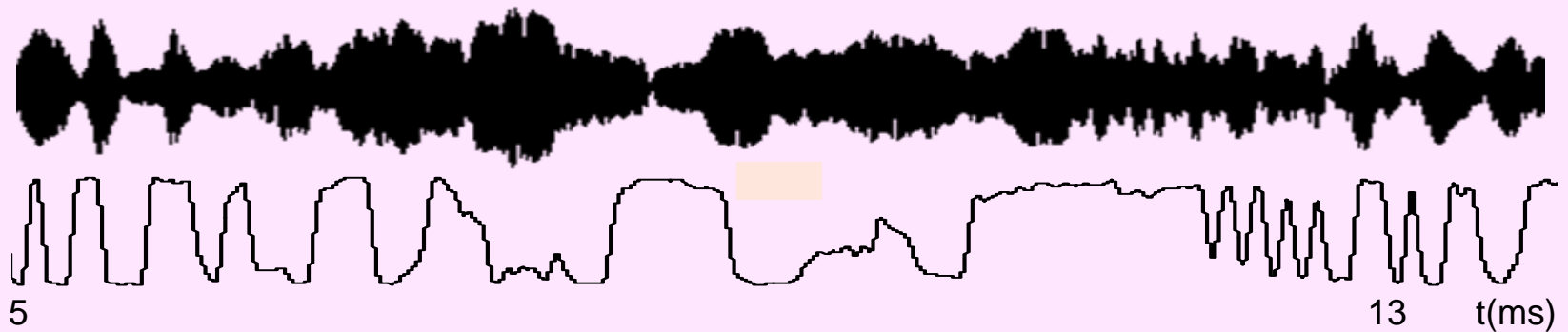
Top: Input signal - Bottom: Hilbert Transform Phase-Detector Output
