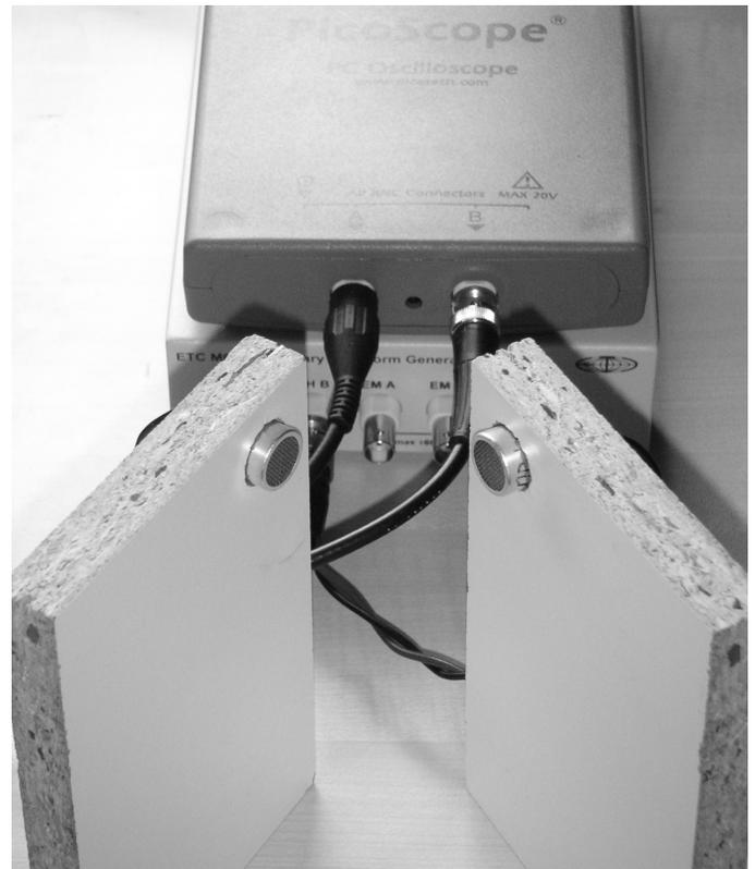
Figure 2. Experimental set-up: Two 40 kHz air-transducers, one arbitrary waveform generator (ETC M631), one PC oscilloscope (PicoScope® 3223)
