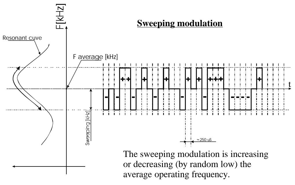
$F_{operating}[kHz] = F_{average}[kHz] + /- Sweeping[kHz]$
