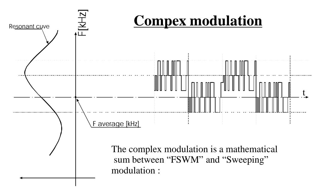
F<sub>operating</sub> [kHz] = F<sub>average</sub>[kHz] + FSWMRange[kHz] +/- Sweeping Range[kHz]
