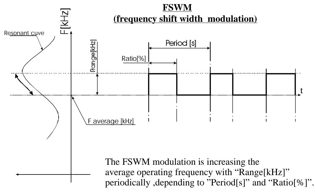
$F_{operating}[kHz] = F_{average}[kHz] + Range[kHz]$
