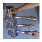
• 3 Party Transducers: Our MMM generators offer great flexibility in adapting to other supplier's transducers or ultrasonic baths. We can make inductive and frequency adjustments in the field to turn ordinary ultrasonic baths into super cleaning systems.
