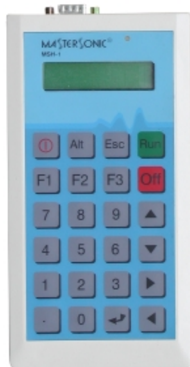
Fig. 4. Remote Control Panel
