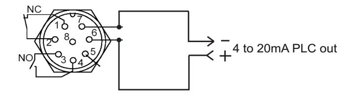
The connection to the 4 to 20mA output of the PLC is as it is shown on the picture above, or if the output is 0 to 10V, as it is shown on the picture below. A external resistor 510 ohms is required.
