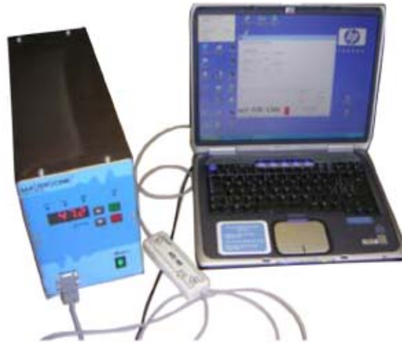
Fig. 3.2. Generator Control using the PC serial port. Connection method.
