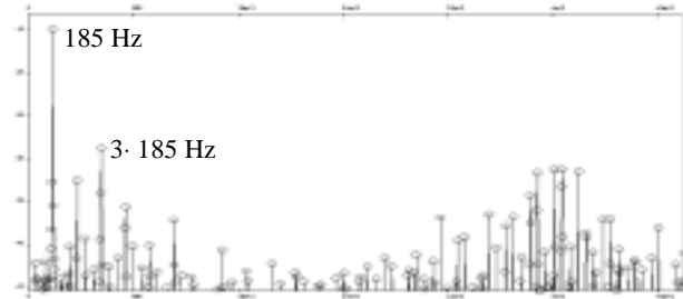
Figure 6 : Power Spectrum at OBBQC output in 2 tone test
