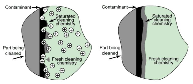
Ultrasonic cavitation and implosion effectively displace the saturated layer to allow fresh chemistry to come into contact with the contaminant remaining to be removed. This is especially beneficial when irregular surfaces or internal passageways are to be cleaned.
