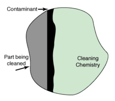
In removing a contaminant by dissolution, it is necessary for the solvent to come into contact with and dissolve the contaminant. The cleaning activity takes place only at the interface between the cleaning chemistry and the contaminant.
