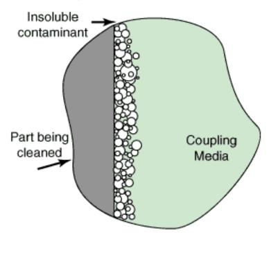
Some contaminants are comprised of insoluble particles loosely attached and held in place by ionic or cohesive forces. These particles need only be displaced sufficiently to break the attractive forces to be removed.
