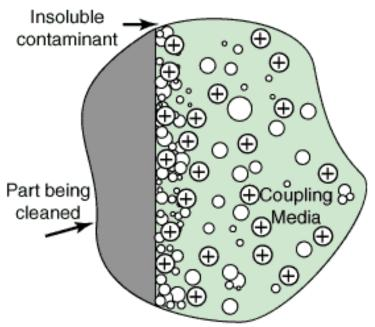
Cavitation and implosion as a result of ultrasonic activity displace and remove loosely held contaminants such as dust from surfaces. For this to be effective, it is necessary that the coupling medium be capable of wetting the particles to be removed.
