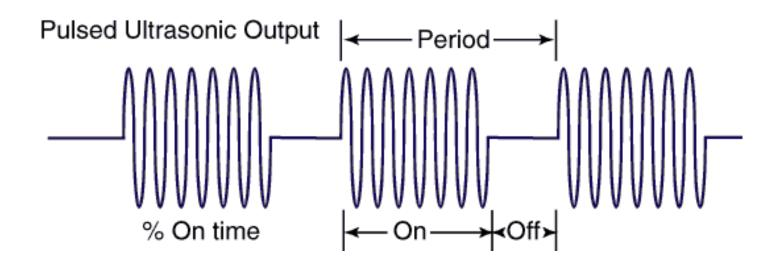
The percentage of time that the ultrasonic energy is on may also be changed to produce varied results. At slower pulse rates, more rapid degassing of liquids occurs as coalescing bubbles of air are given an opportunity to rise to the surface of the liquid during the time the ultrasonic energy is off. At more rapid pulse rates the cleaning process may be enhanced as repeated high energy "bursts" of ultrasonic energy occur each time the energy source is turned on.
