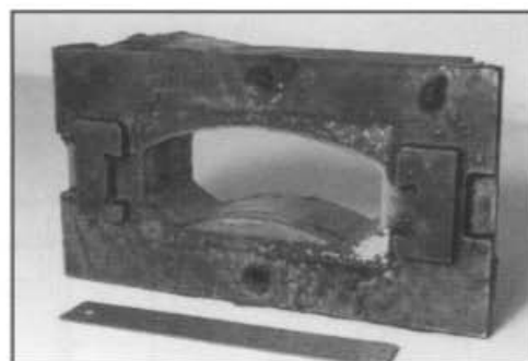
Figure 1. Note encrusted material on mold surface.
