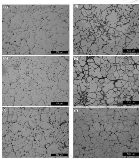
Effect of liquid temperature on the microstructure after casting Al-Mg-Mn: (a-c) with 1kg/ton of Al5Ti1B; (d-f) with MMM Ultrasonic Technology. (a) and (d) casting at 700C; (b) and (e) casting at 685°C; (c) and (f) casting at 670°C.
