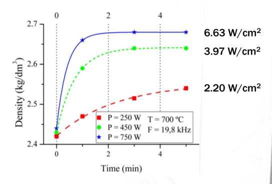
Effect of temperature and ultrasonic power in Al-Si-Cu processing
