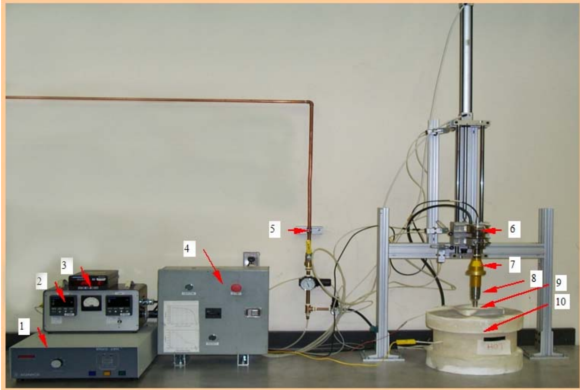
Fig. 4.1. Experimental system for ultrasonic degassing of aluminum in air. Key: (1) ultrasonic generator; (2) controller for electric furnace; (3) melt temperature indicator; (4) pneumatically operated device; (5) air inlet; (6) transducer; (7) booster; (8) horn; (9) radiator; (10) electric furnace.
