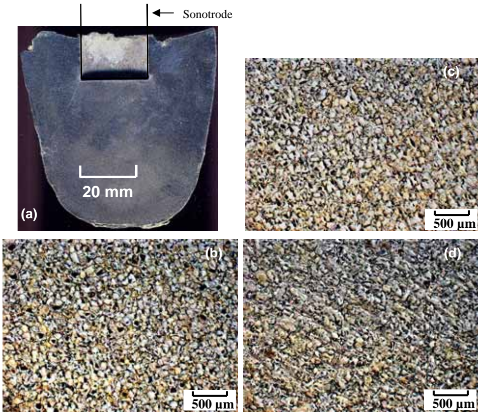
Fig. 5. Grain structures of an AZ91 ingot sample solidified under ultrasonic irradiation at a nominal intensity level of 1700 \text{ W cm}^{-2} . The insertion depth of the sonotrode was \sim 20 \text{ mm} . Micrographs (b), (c) and (d) were taken from 5 mm, 15 mm and 45 mm below the sonotrode radiating face, respectively (Ramirez & Qian, 2007).
