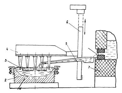
*Figure 1.* Schematic of large-scale ingot casting of aluminum alloys with ultrasonic processing of molten metal in the liquid bath: 1, ingot; 2, liquid bath; 3, distributing (casting) trough; 4, ultrasonic transducers; 5, casting tray; 6, moving mechanism for ultrasonic sources; and 7, holding furnace containing molten metal.
