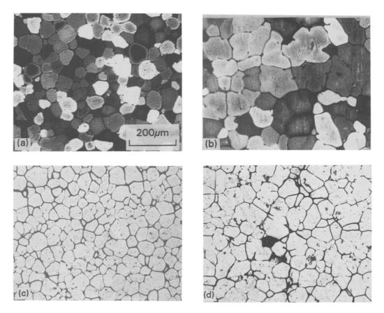
*Figure 5.* Grain structure of 1973 (0.3% Zr) ingots 270 mm in diameter (a,  $b \times 100$ ) and intermetallic particles (c,  $d \times 100$ ) in a standard process (b, d) and after the following treatment of the molten alloy: F + T + UST-2 (a, c).
