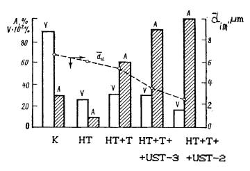
*Figure 3.* Effect of ultrasonic processing of molten metal in combination with other kinds of treatment on the structure of 1973 (0.3% Zr) ingots 145 mm in diameter (see explanations in text).
