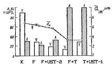
*Figure 4.* Effect of fine filtration (Usfirals-process) using multilayer screen filters (F) combined with other kinds of molten metal treatments on structure of 1973 (0.3% Zr) ingots, 270 mm in diameter (see explanations in text).
