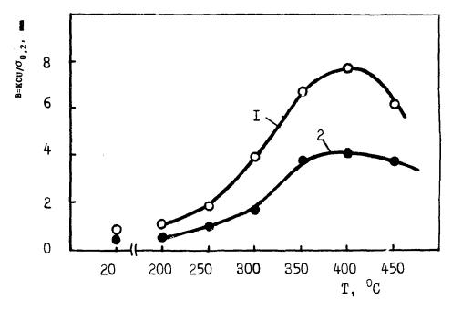
*Figure 2.* Effect of nondendritic structure on ductility in the hot-deformation temperature range (B = KCV/0.2% YS), where KCV is the impact toughness). Data for an ingot 830 mm in diameter from a 1973 grade alloy (Al-Zr-Mg-Cu-Zr) with 0.15% Zr: 1, casting with ultrasonic processing (nondendritic structure) and 2, casting without ultrasonic processing (dendritic structure).
