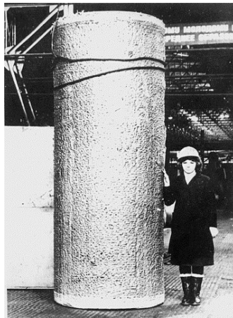
Figure 5.1 A billet with non-dendritic grain structure produced using UST (an AA2324 alloy, diameter 1200 mm, weight 10 t) [8, 10].
