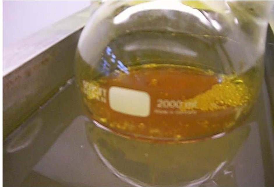
**Minerals with precious metals content in glass vessel with acids mixture. MMM ultrasonic processing switched ON and OFF (see the difference in extracting activity)**
