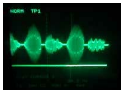
Oscilloscope signal of the multiple-modulated output, load signal in the low frequency domain (carrier is not visible)
