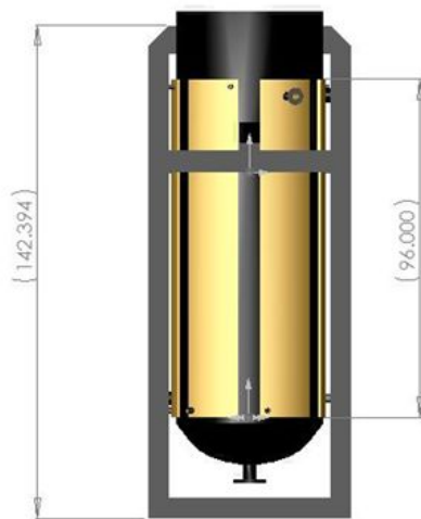
15 kW acoustic load (Extractor: H = 3.6 m, OD = 1 m)
