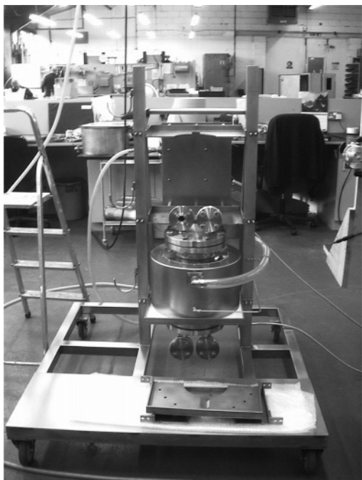
Figure 9. C 3 Technology ultrasonic flow cell: 5-L cell fabricated in Hastelloy for pharmaceutical use with two inputs and two output flanges for flexible hose attachment.
