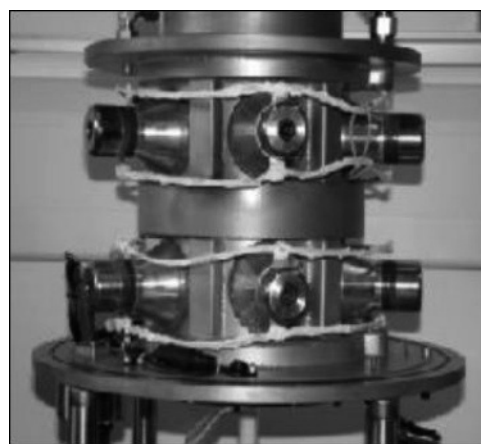
Figure 8. C 3 Technology ultrasonic flow cell: 5-L cell in stainless steel with bonded transducers shown with acoustic shield removed for clarity.
