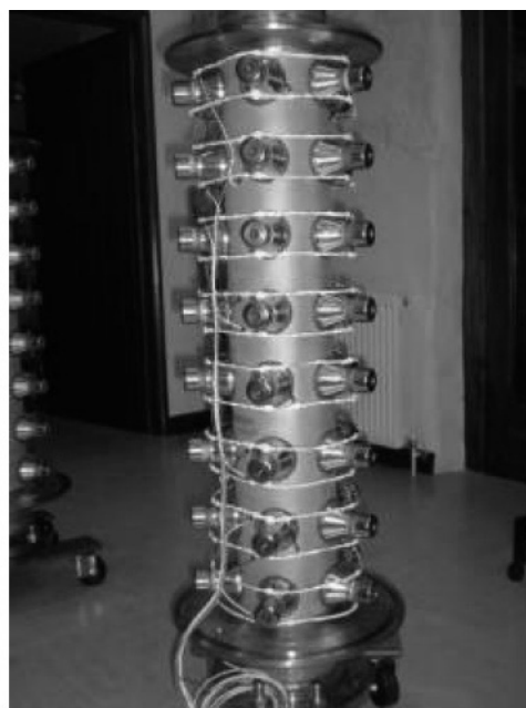
Figure 10. C 3 Technology 20-L flow cell fabricated in hard chrome-plated stainless steel with 40 bonded transducers for use in the alumina industry; shown with acoustic shield removed.
