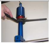
Pictures presenting ultrasonic converter with water jacket (upper part), wave-guide (middle part) and aluminum clamps on the reactor tube (bottom). Apply fastening of clamps, slowly, symmetrically and gradually (on both sides) until reaching **30 Nm torque** value (use proper torque wrench; -not presented on the pictures here). For fixation (screwing, unscrewing) of converter and wave-guide use here presented wrenches.
