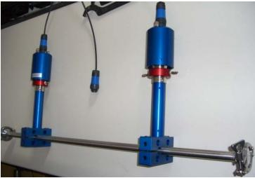
In operation, the biggest care should be taken to keep constant low temperature on ultrasonic converters (always below 50 degrees Celsius). Water jackets should be connected to a cold water flow in order to keep aluminum wave-guide cold and to
