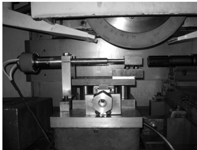
Fig. 1. (a) Scheme of the experimental set-up. (b) Experimental set-up for ultrasonic assisted dry grinding.
